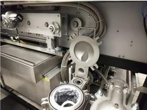
Stainless steel machine components with easy roll-out filtration
