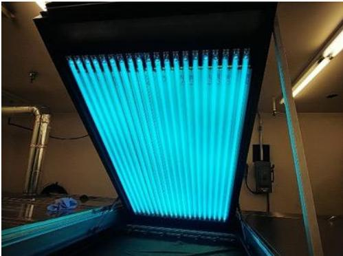
Inline-UV post-exposure ensures high plate uniformity
